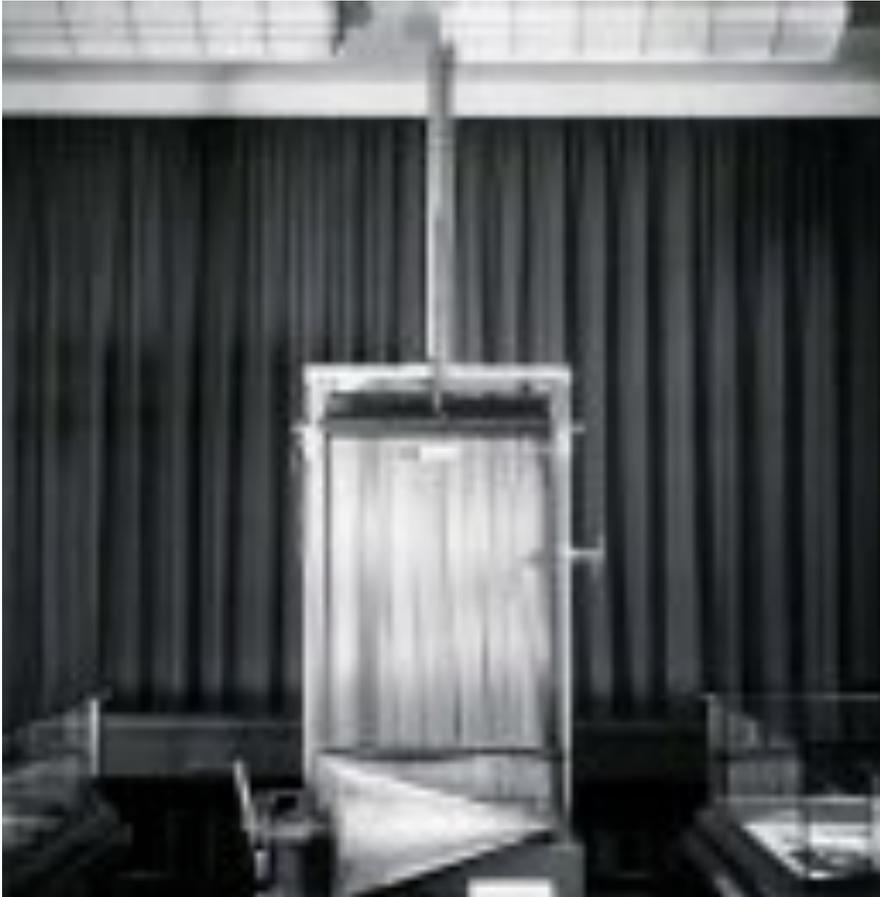
**The Michelson-Stratton harmonic analyzer, one of the first mechanical analogue computers, recorded data from spectroscopic experiments.**
